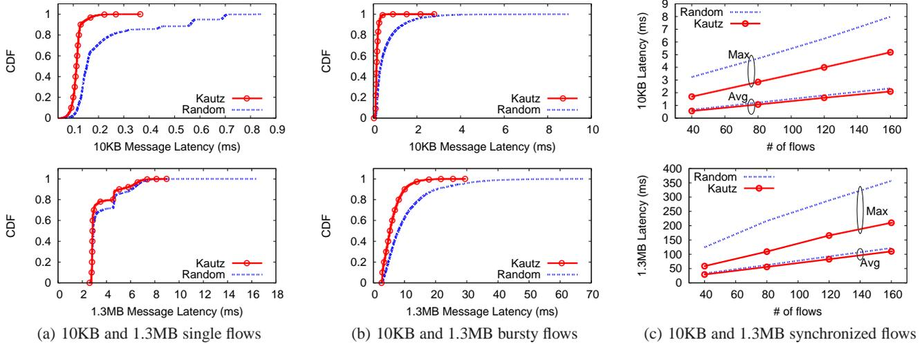
**Figure 12: Angora’s end-to-end TCP delay performance when carrying 10KB (top) and 1.3MB (bottom) messages. (a) CDF of single flow latency. (b) CDF of per-message latency of the two bursty flows. (c) The maximum and average per-message latency of multiple synchronized flows.**
