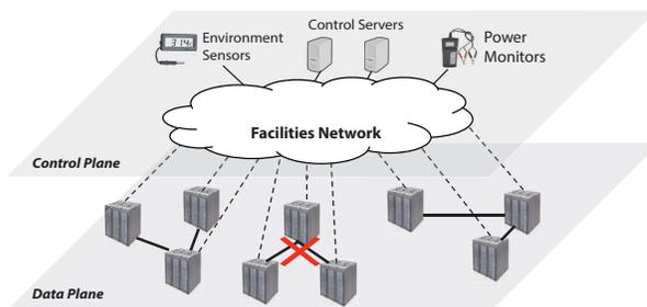
Figure 1: A facilities network providing robust delivery of control traffic in a data center.
